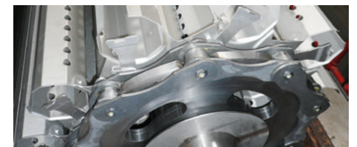
Stainless steel chain for sterilizing vegetables, frozen food, and pet food.
